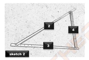
Assemble brackets 2, 3 and 4, formatting a triangle as shown on sketch 2.
