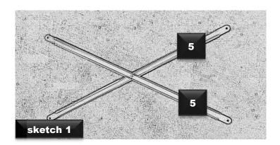
Assemble the two brackets number 5 as an X using the bolt and nut provided through the middle hole.
